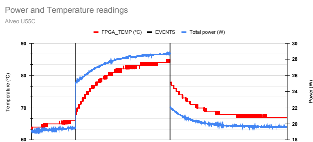
Figure 6: Temperature vs Power Consumption in Alveo U280.
